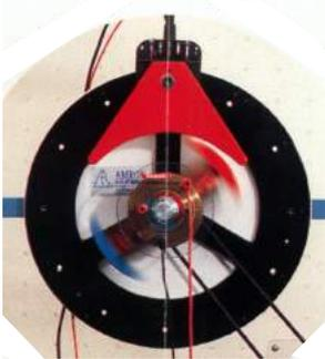
A two pole rotor is energised from DC supply via a pair of sliprings. A galvanometer connected to the field coil indicates the current induced in the coil during manual rotation of the rotor.
