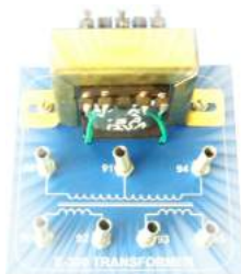
Individually mounted transformer
