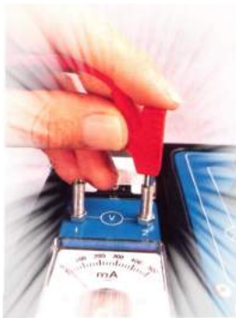
Springs accept 4mm banana plugs
