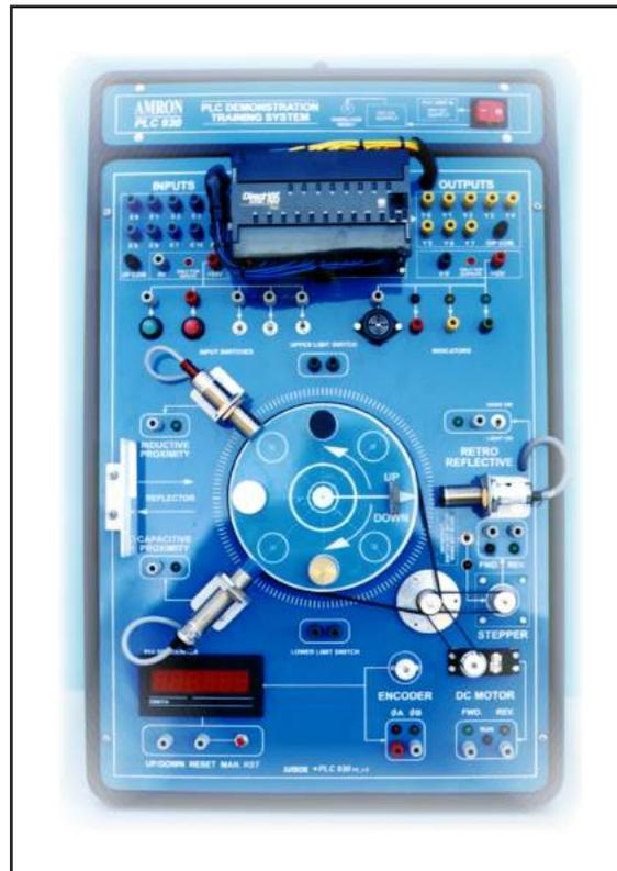
The PLC 930 has been designed to complement the PLC 910 Student Trainer. Whereas the 910 deals with PLC-managed control of working devices where position is not important, the 930 incorporates a DC motor with encoder to render information about speed, direction and position.
