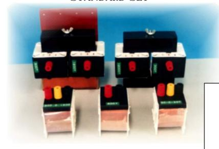
The AEM 100 is a set of demountable transformers that enable the student to construct a number of inductive devices with various combinations of turns-ratios and then study such parameters as the relation between input and output voltages, primary and secondary currents, prove Farady's law of induction, etc.
